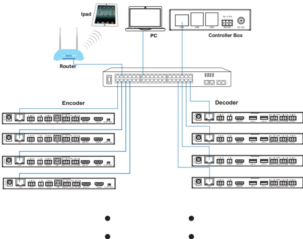
**Step 2:** Set the ipad's IP address to the same network segment with Switch, for instance set PC IP address to 192.168.1.30 and Subnet mask to 255.255.255.0.
