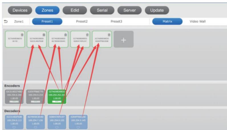
You can also drag Encoder into the frame of ALL RX, so that you can match an Encoder video signal to ALL Decoders, as shown in the following figure:
