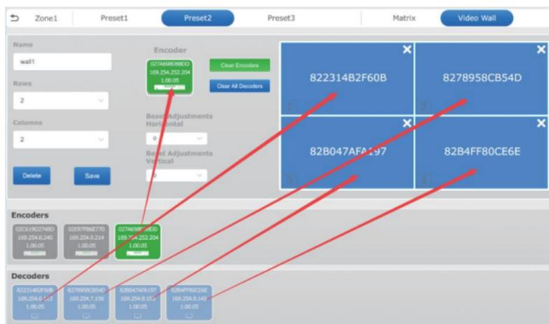
A 2 \* 2 video wall setting is composed, and a maximum wall of 4 \* 6 can also be set. If you need to delete this wall, just click the “Delete” button.
