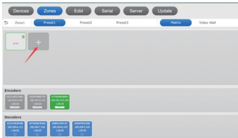
Click the + button to built new correspondence. Drag a Decoder to the corresponding frame, then drag the required Encoder to the same frame, as shown in the following figure.
