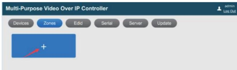
Click the + button to create new zones, and you can create no more than 16 zones. Each zone can set different application methods **matrix / video wall**.
