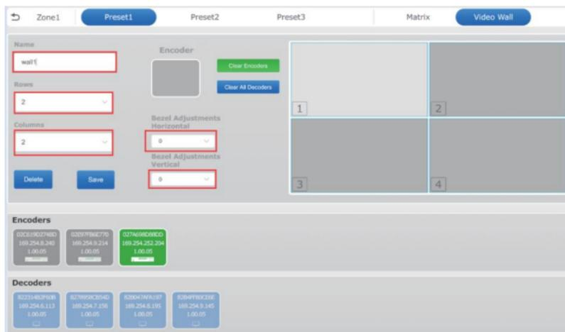
You can set the wall's name, rows, columns and Bezel adjustments. After completing the settings, click "Save" to save the configuration, or click "Delete" to delete.
