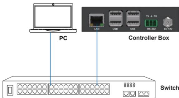
Figure 2. Connect the Controller with PC via the LAN port
