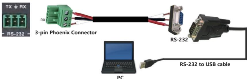
Figure 1. Connect the Controller with PC via the RS-232 phoenix connector
