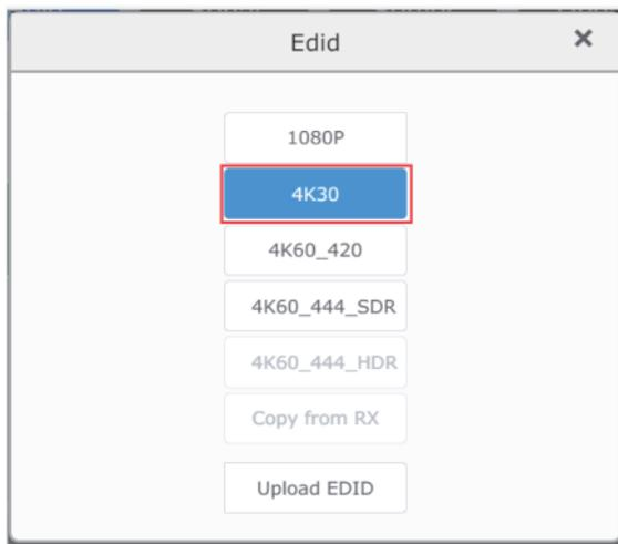
As shown in the figure, there are 7 types of EDID. When the Encorder has a connection relationship, you can choose “Copy from RX (Decorder)”. Another type is Upload EDID.
