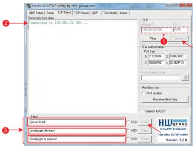
**Step 3:** Input the IP Address (169.254.23.100) and Port number (6008) of the Controller box at “label 1”, and then click the “Connect” button. PC will try to connect the Controller as shown in “label 2”.
