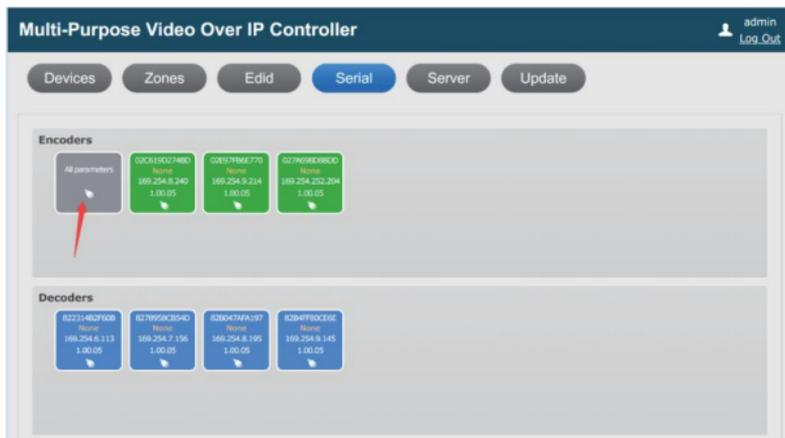
Click the arrow pointing icon to configure the RS232 parameters of all Decoders and Encoders in this system. The interface after clicking is as follows:
