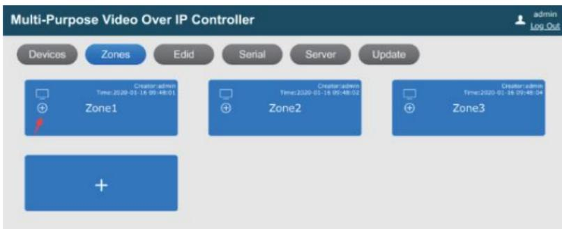
Click the + button to add Decoders for the zone, as shown in the figure below. After being selected, the Decoder will be in the corresponding zone.
