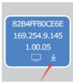
As shown in the figure above, click the arrow pointing icon in the Decorder frame to save the EDID of the display device connected to Decorder, and then you can upload the saved EDID on Encorder to Source.
