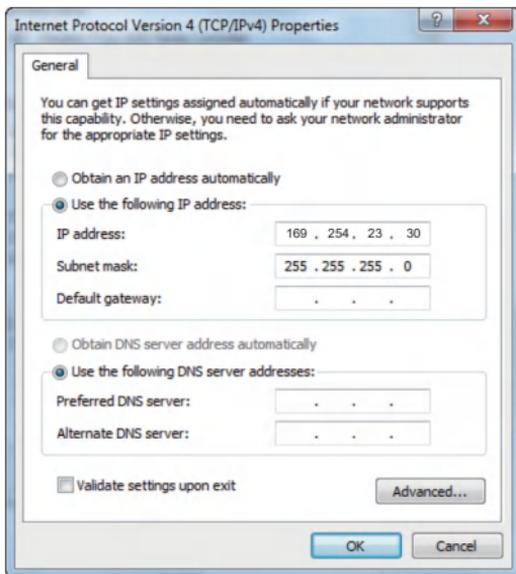
**Notice:** The IP address of the PC, Controller and other IP products should be in the same network segment. As the Controller’s IP address is 169.254.23.100, the computer’s IP should be set 169.254.23.X (X contains 1~255 except 100).
